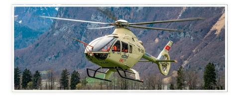
Kopter's latest AW09 prototype, designated PS4 and featuring the new Safran Arriel 2K engine, performed its maiden flight in Mollis, Switzerland on the 16th March 2023. This flight lasted 20 minutes and successfully completed all set objectives, performing hovers at low altitude, spot turns, straight and sideways flights up to 20 knots as well as several landings and take-offs.
